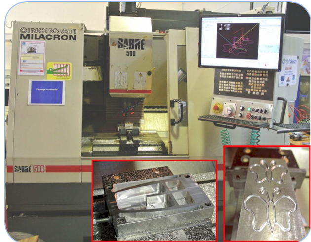
Figure 5: Milling with LinuxCNC [EC-Nantes]
